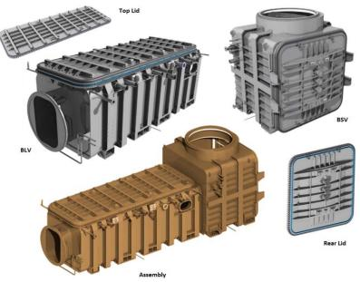
Main welded assemblies of the Neutral Beam Vacuum Vessel.
